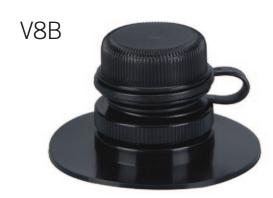
They are the classic lightweight and economical valves for Kite and Wing, available with base in PVC or TPU so that they can be easily welded or glued onto the bladder. The outer diameter of the welding flange is 55 mm.
